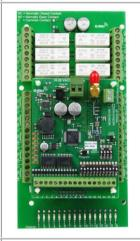
MCR91512SS 12-Channel 915MHz Receiver with Open Collector Output
