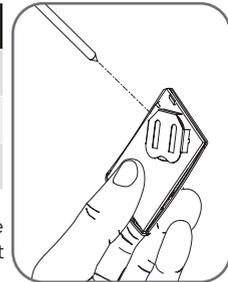
2. Use finger nails to separate the remote casing to expose circuit board.
