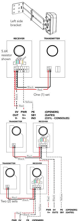
**NOTE:** Mount the receiver on the side of the doorway / gateway closest to the opener / console.
