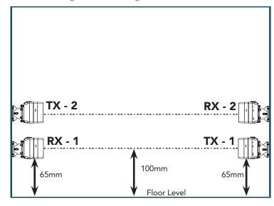
a. ATA recommends the transmitter and receiver are placed in line of sight, with the beam 100mm above the ground level (as per AS60335). This can be achieved by ensuring the bottom of the receiver and transmitter are 65mm above ground level. They should also be placed as close as possible to the door / gate opening.In industrial applications it is recommended that multiple Safety Beams are fitted.
