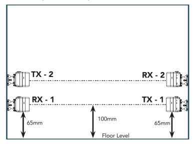
ATA recommends the transmitter and receiver are placed in line of sight, with the beam 100mm above the ground level (as per AS60335). This can be achieved by ensuring the bottom of the receiver and transmitter are 65mm above ground level. They should also be placed as close as possible to the door / gate opening. In industrial applications it is recommended that multiple Safety Beams are fitted.
