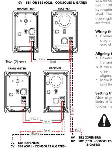
NOTE: Mount the receiver on the side of the doorway / gateway closest to the opener / console.
