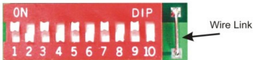
Make sure the 10 DIP switches of the transmitter board matches the first 10 DIP switches of the receiver. Set the receivers dip switch 11 and 12 as described above.
