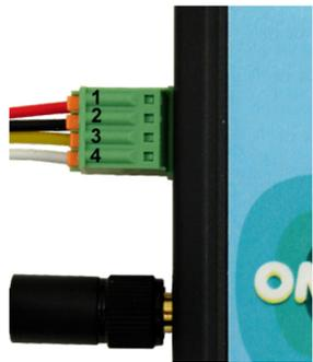
**PINS 1 & 2** Power supply input, not polarity conscious.
