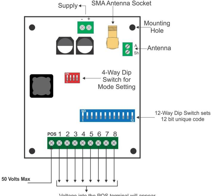
Voltage into the POS terminal will appear on these terminals when the channel is activated. Max recommended switching current is 120 mA For higher switching current please see the datasheet for A2982LW
