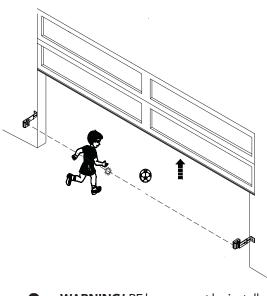
**WARNING!** PE beams must be installed if the closing force at the bottom edge of the door exceeds 400N (40kg force)
