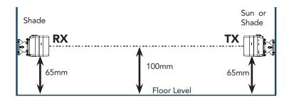
The Safety Beam Kit provides additional safety by preventing the door closing when the beam is blocked by a car, child etc.
