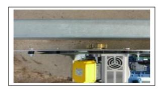
Fix rack to the gate frame keeping 1mm-2mm clearance between the rack teeth and Pinion wheel
